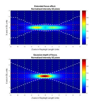
Our <u>small Top Hat beam shapers</u> have many applications, including their use as elongated focus elements for depth of focus extension in transparent materials. However, it turns out that their depth of focus extension is a highly useful even in ablation of non transparent materials such as copper.
