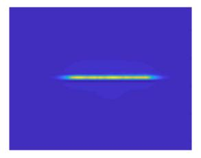
By tailoring the diffuser to the laser, we can make sure the line width remains almost the same s as the original spot size, while significantly improving the top- hat diffuser uniformity.
