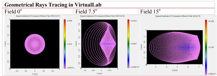
Geometrical raytracing shows spot size is Diffraction limited for tested scan angles.
