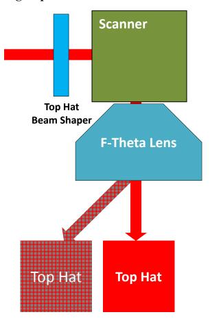
The Top Hat beam shaper is placed before the scanner at some arbitrary distance, as distance doesn't influence functionality. The main concern is for clear apertures within the scanner and F-Theta to be more than ~2.2x incident beam size.
