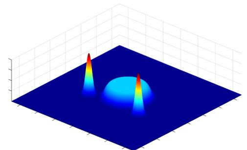
For this purpose, Holo/Or has developed a special homogenizer element that creates 2 small leading rays for cleaning/preheating and 1 large uniform beam that equally distributes the energy over the brazing wire to achieve better melting.
